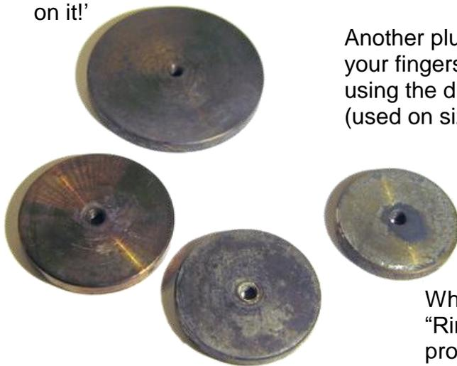
Another plus is that the mandrel size (part that you have in your fingers) is thick (starting at 3mm up to 5mm). When using the disc on a mandrel it will stay perfectly straight (used on size 2mm it can tip over).
