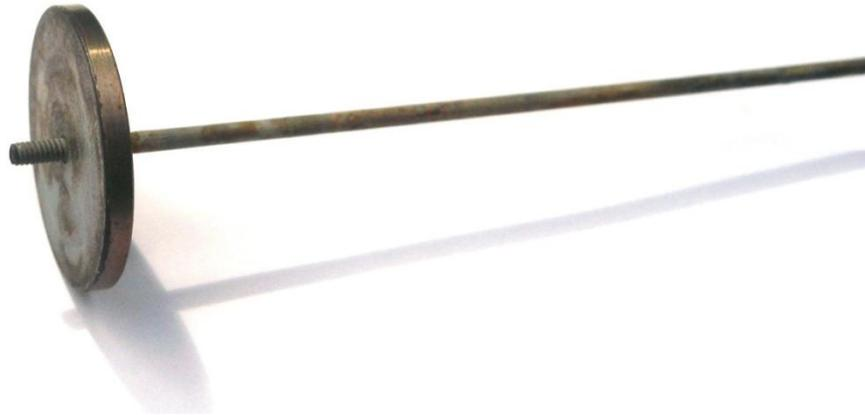
**Step 2** Dip the spoke and disc in bead release (use a wide bottle so you do not touch the edge of the bottle) Air dry the bead release
