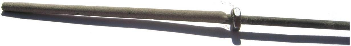
**Step 3** When the bead release is really dried you can push the nut up the spoke. Leave a part of the spoke with bead release above the nut so the screw of the ring won't damage your topper!
